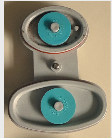
Figure 2: Black particles concerning for mold around the valve in the EZChange module where moisture-containing gas leaves the absorbent canister.
