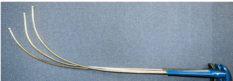
Figure 2: Comparison of single-use stylet with two reusable stylets showing varying degrees of curvature deformation.
