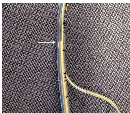
Figure 4. Endotracheal tube patency. Multiple 2.5 endotracheal tubes were found not to allow for passage of a size 5/6 French suction catheter. This appears to be due to a manufacturing defect where the pilot line inserts into the endotracheal tube (arrow).
