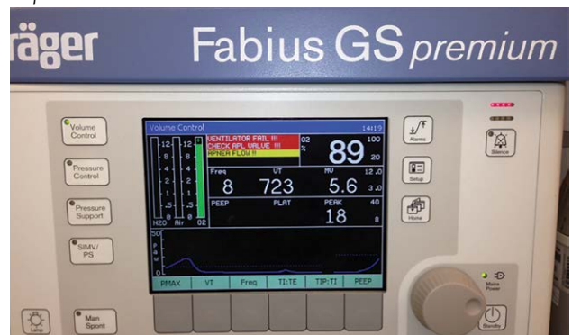
Figure 2. Despite the ventilator alarms, there was no loss of tidal volumes, and the ventilator appeared to function appropriately. The alarms continued—even after resumption of manual ventilation. Close inspection revealed a small cut in the APL valve bypass tubing as the source of the problem.
