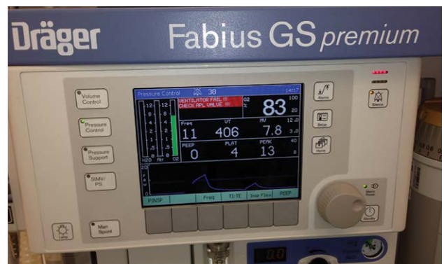
Figure 1. The authors successfully performed the anesthesia machine checkout on the Dräger GS Premium machine prior to anesthesia induction. At the initiation of mechanical ventilation, despite the machine passing checkout, the machine alarms sounded for “Ventilator Failure!!!,” “Check APL Valve!!!,” “Apnea Pressure!!!”
