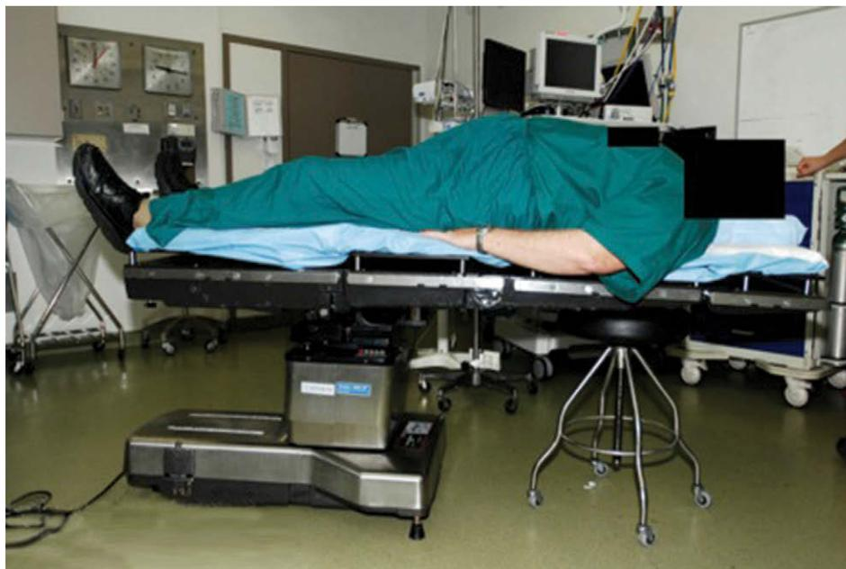
Figure 1: We enlisted the help of a colleague who weighs 160.3 kg to demonstrate the danger of OR table tipping on the Amsco 3085 SP surgical table when used in reverse orientation. Upon releasing the floor locks (with safety support present), the table tipped instantaneously.
