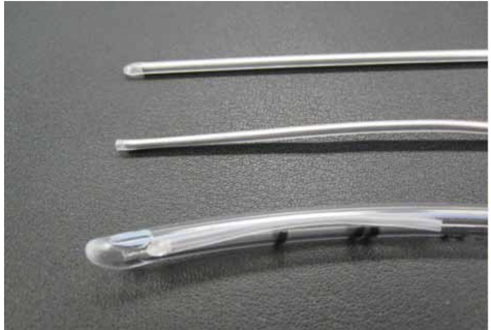
Figure 1: From top to bottom: Intact stylet; stylet immediately after distal end sheared off; sheared off tip in endotracheal tube.
