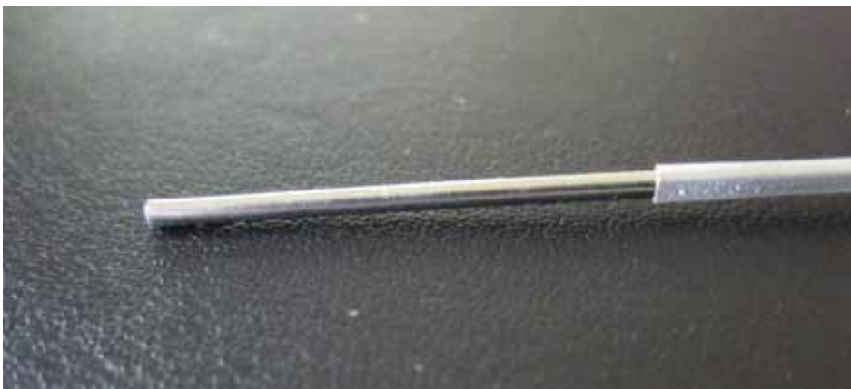
Figure 2: Stylet after plastic covering retracted.
