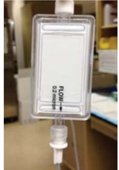
Figure 5. Open system demonstration: Note prime level decreasing inside filter housing. This happens while the fluid drips out at the open end.
