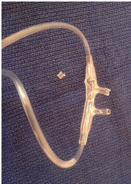
Figure 1. Ruptured Nasal Canula.
