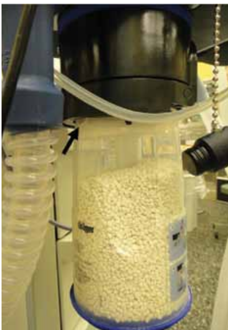
Figure 1: The defective CLIC absorber. A) The canister in place on the machine. The black arrow points to the defect. B) A close-up of the hole.
