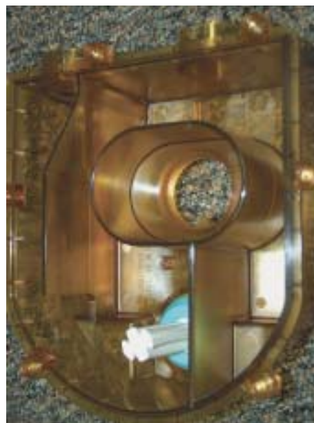
Photo 1. Bottom view of the active scavenging reservoir without valve (correct configuration).
