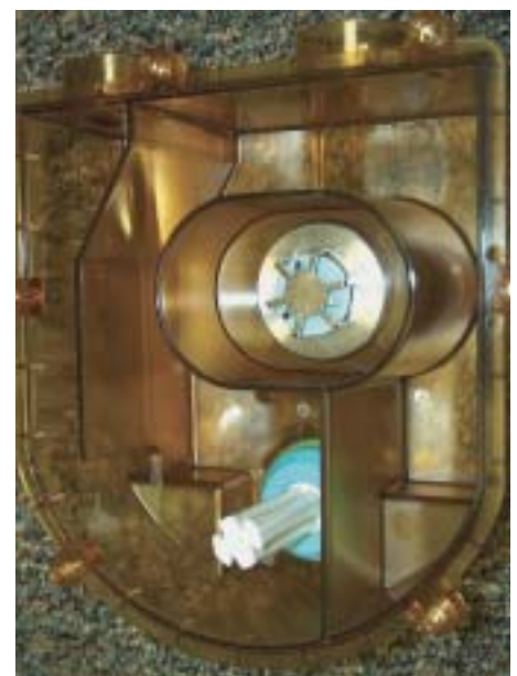
Photo 2. Bottom view of the active scavenging reservoir with valve in place (incorrect configuration).
