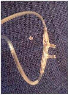
Figure 1. Ruptured Nasal Canula.
