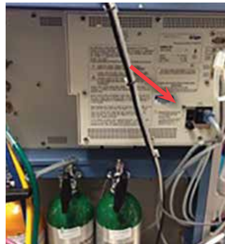
Figure 4: Fabius On/Off Switch (back of machine).
