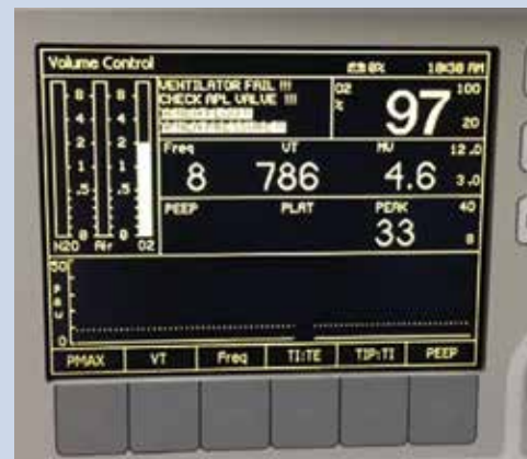
Figure 1. Screens displayed on Dräger Apollo and Fabius GS anesthesia machines at time of battery failure.
